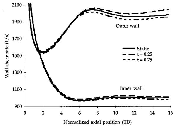
**FIGURE 4.** Wall shear rate vs normalized axial position at the inner and outer walls for the static (mean radius of curvature) and dynamic cases at the same two time points shown in Fig. 3. For reference, the shear rate in an equivalent, fully developed, straight tube flow would be  $1067 \text{ s}^{-1}$ .
