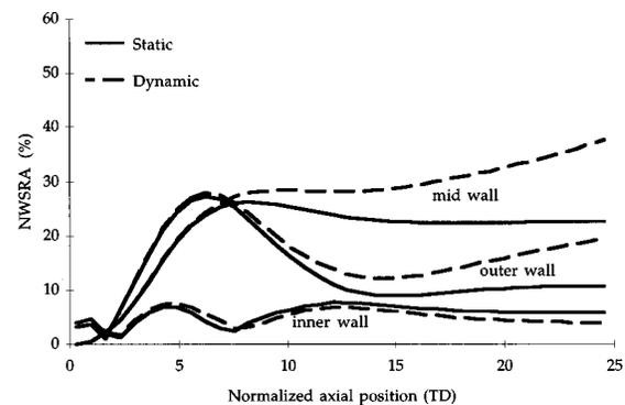
**FIGURE 6.** NWSRA vs axial position for  $\delta_m=0.03$  and  $\varepsilon=0.5$  at the inner, mid and outer walls. The NWSRA is higher at the mid and outer walls. The dynamic and quasistatic predictions were approximately the same within the first 10 TDs.
