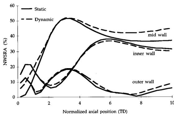
**FIGURE 8.** NWSRA vs axial position for  $\delta_m=0.12$  and  $\epsilon=0.5$  at the inner, mid and outer walls. The highest NWSRA noted in this study, 52%, was found at the midwall in this case. The dynamic and quasistatic predictions were approximately the same within the first 10 TDs.
