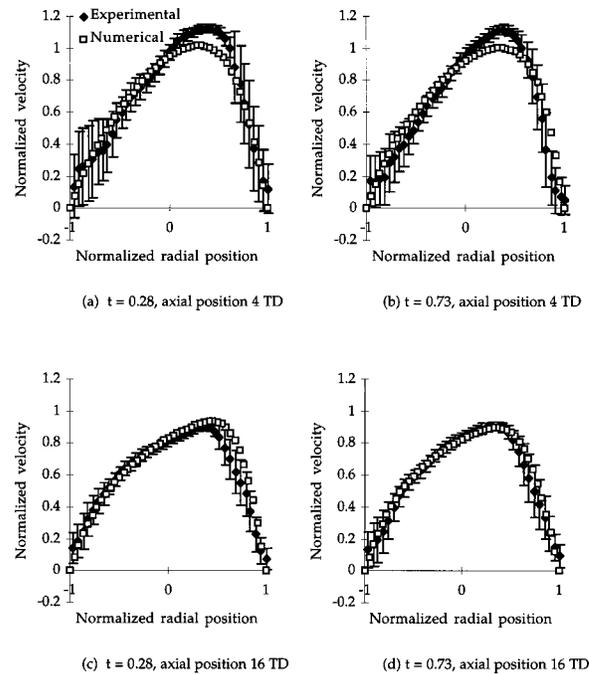
**FIGURE 9.** Comparison of the experimental and computational velocity profiles at (a) and (b) 4 TDs and (c) and (d) 16 TDs at two different time points in the simulated cardiac cycle. The correlation coefficient that resulted from comparing the experimental to the computational results at all positions and time points was 0.93.
