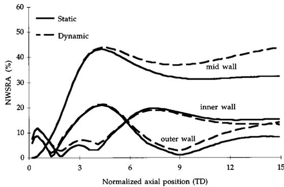
**FIGURE 7.** NWSRA vs axial position for  $\delta_m=0.08$  and  $\epsilon=0.5$  at the inner, mid and outer walls. The NWSRA is higher at the midwall. The dynamic and quasistatic predictions were approximately the same within the first 10 TDs.
